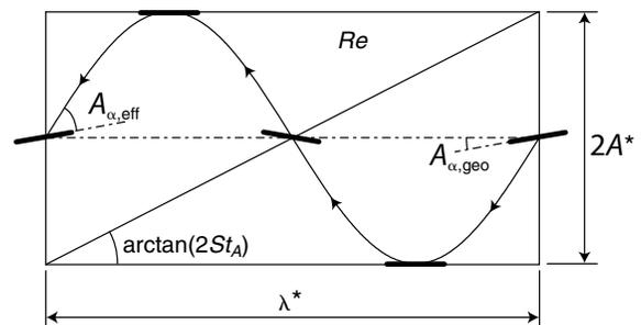
Fig. 1. A graphical representation of the non-dimensional parameters of a sinusoidally flapping foil: dimensionless wavelength  $\lambda^*$ , amplitude ratio  $A^*$ , amplitude-based Strouhal number  $St_A$ , geometric angle of attack amplitude  $A_{\alpha,geo}$ , effective angle of attack amplitude  $A_{\alpha,eff}$ , and stroke-averaged Reynolds number  $Re$ .
