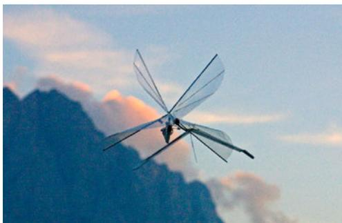
**Fig. 1** DelFly, a flapping wing micro aerial vehicle inspired by insect flight with slack sail-like wings [3]
