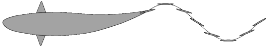
Fig. 1 The tail (caudal fin) of a thunniform swimmer (e.g., tuna and many sharks) forms the main source of propulsion. The tail can be effectively approximated as a heaving and pitching foil
