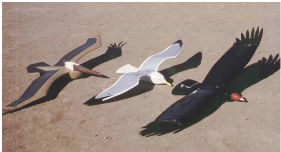
Figure 8. These elegant models of a pelican, sea gull, and a turkey vulture can soar stable without a vertical tail. Image credit: Robert Hoey.
