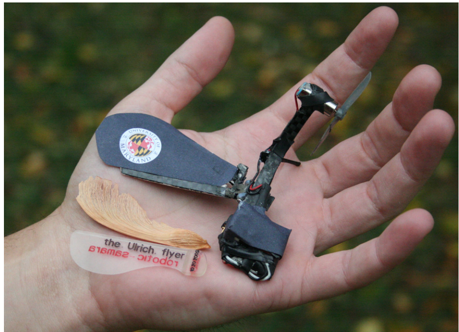
Figure 9. At scale robotic maple seed. Image credit: Evan Ulrich.
