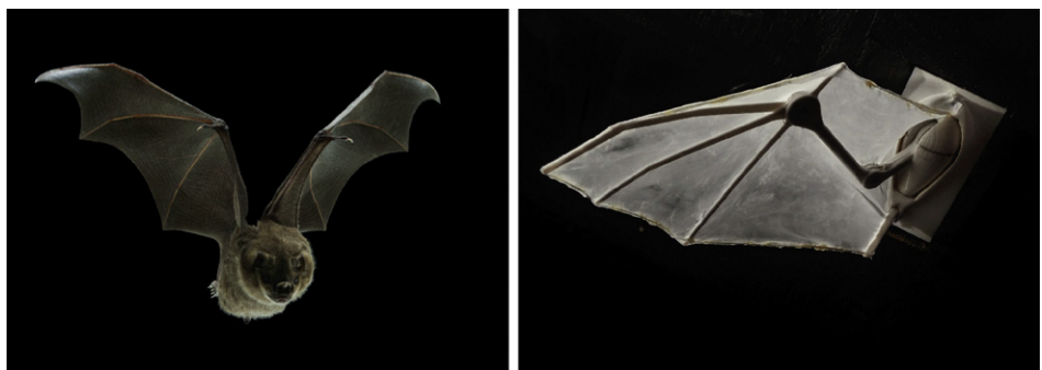
Figure 6. Bat Artibeus jamaicensis flying in the Brown bat flight wind tunnel (left) and bat-inspired flapping robot tested in the same wind tunnel (right). Photo credit: Sharon Swartz and Kenny Lab at Brown University.
