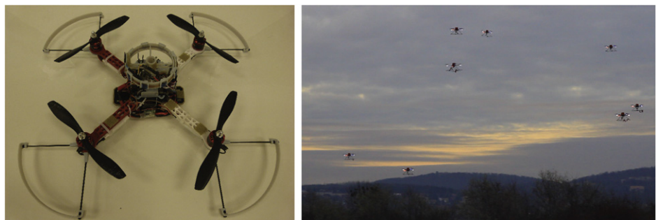
Figure 9. Quadcopter equipped with insect vision algorithms to avoid obstacles (left) and a swarm of quadcopters controlled by an algorithm-inspired by pigeon flocking (right). Photo credit: J Keshavan (left) and Csaba Virágh (right).
