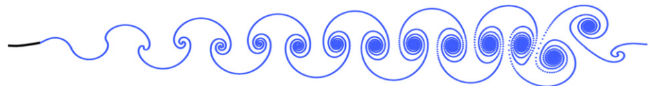
Figure 4. Vortex wake generated by a flapping flexible foil. Image credit: Annika Eberle.
