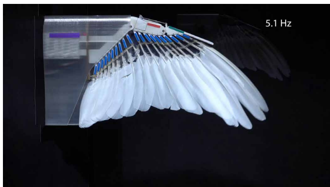
Movie 1. Morphing wing response to increasing flexion/extension cycling frequency under aerodynamic loading. A subset of the cycling frequencies tested (0.4, 1.0, 2.0, 5.1, and 8.9 Hz) shows that the PigeonBot wing responds well to control inputs up to \sim 5 Hz.
