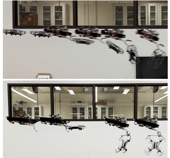
Fig. 1. Composite photo of the grasping sequence. Top: grasping drone moving at 2 m/s catching a moving target drone at 0.5 m/s. Bottom: grasping drone at 2.7 m/s catching a hovering target.
